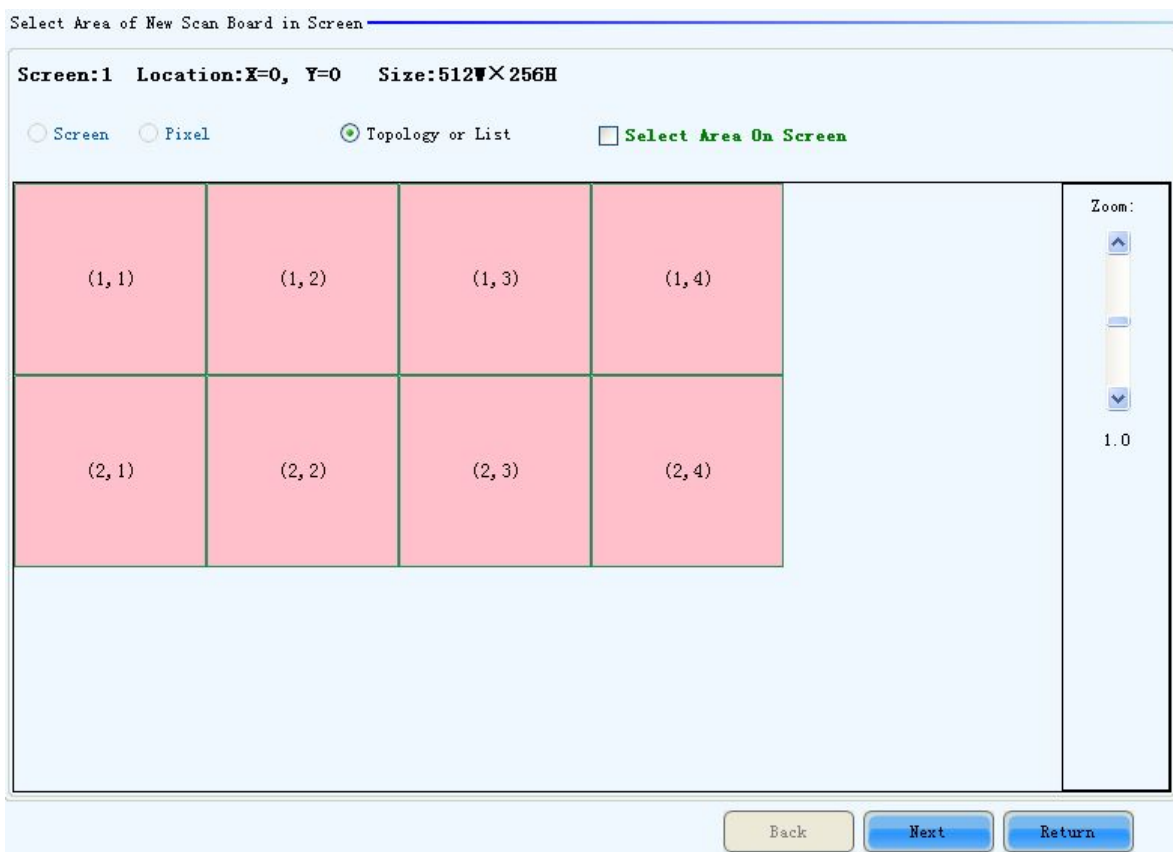
Fig. 5-92 The page for specifying the working area of the new receiver card
